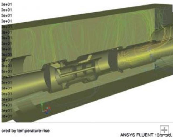
Grid Solutions has continually developed and improved this mechanism. Thanks to the thermally assisted puffer-type technology, it is possible to interrupt short-circuit currents of at least 160 kA with a spring-operating
