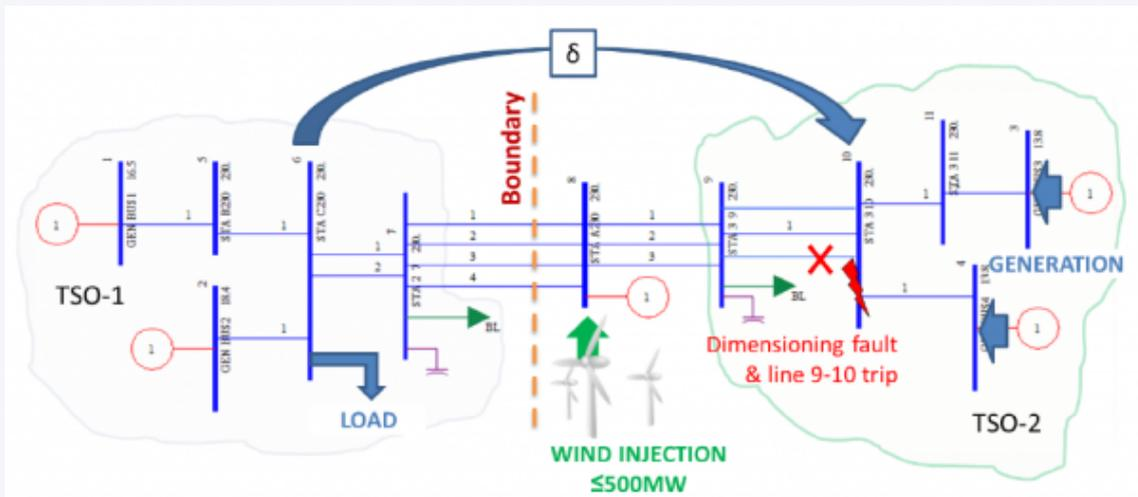
Dynamic model including synchronous generation, a transiently constrained corridor, and wind generation injection.
