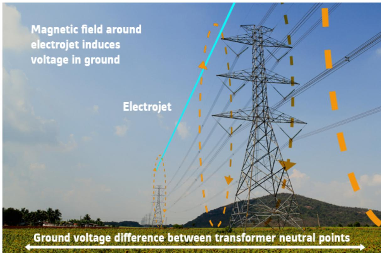
How does this happen? “Due to the local voltage differences induced by the electrojets at the Earth’s surface, a quasi-direct current (DC)—i.e., a current of very low frequency— may flow
