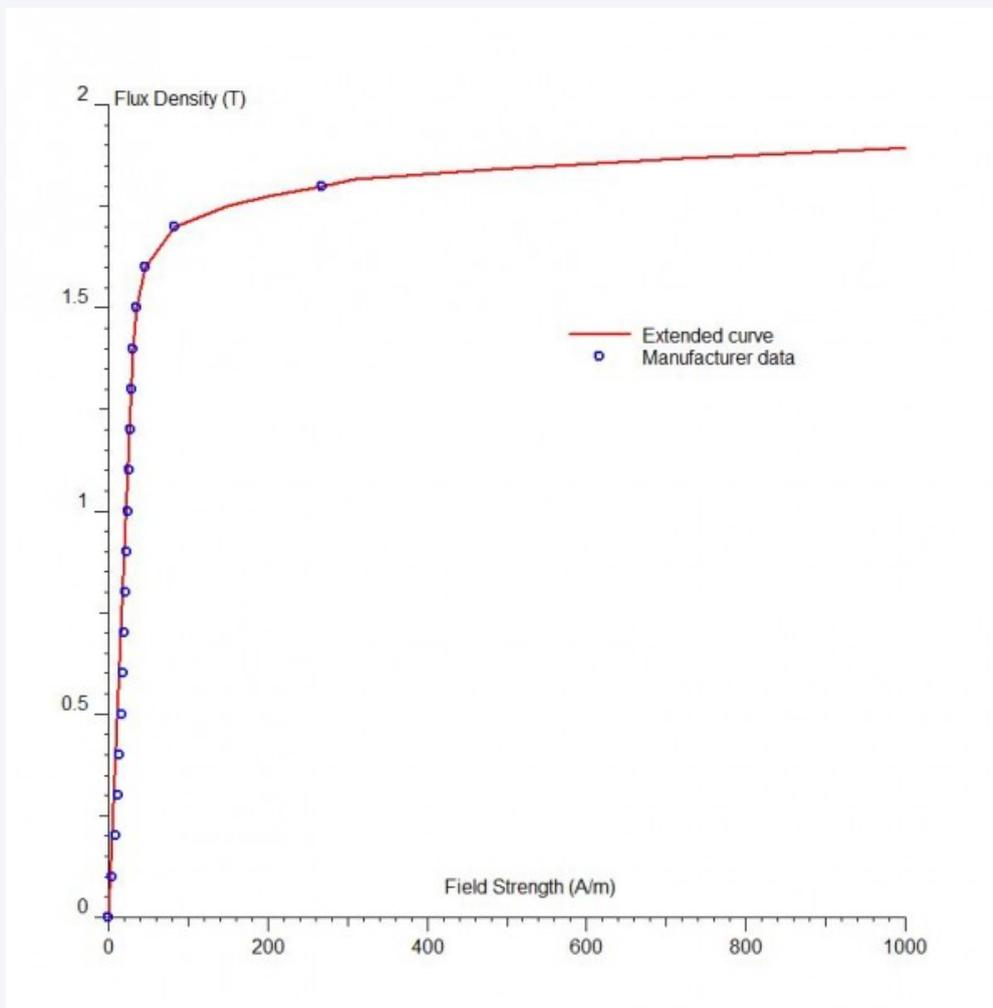
*Magnetization curve for typical transformer steel, showing mathematical extension.*
